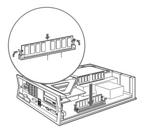
There is only one correct way to insert the memory module. Make sure the rivets of the module are lined up with the connector.
